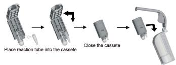
Place reaction tube into the device
