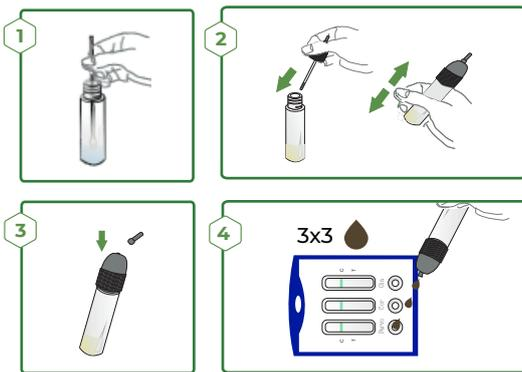
**Note:** If the fluid does not begin to migrate through the test strip, use the cotton swab's upper tip to remove any solid material which may be interfering with the flow.
